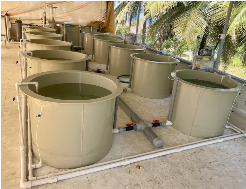
FIGURE 2 Tanks with recirculating aquaculture system (RAS) used for broodstock development of Andaman damsel Pomacentrus alleni .
